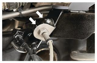
Fig. 3: Mount the reservoir bracket under the brake bracket.
