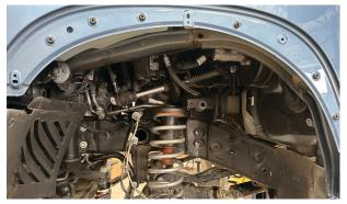
Fig. 1: Pull the fender liner.
