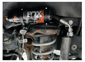
Fig. 6: Mounted Performance Elite Reservoir.
