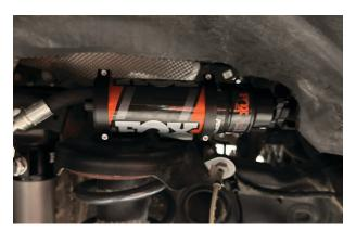
Fig. 9: Example of a cut fender liner.
