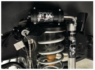
Fig. 7: Mounted Performance Series Reservoir.
